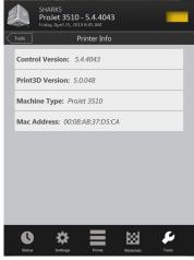
**Printer Info**: provides information about the control software version, Print3D software version, machine type and its address.
