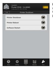
**Printer Shutdown:** Click on the arrow key to shutdown printer. Click the arrow keys to reboot printer or to restart the software.
