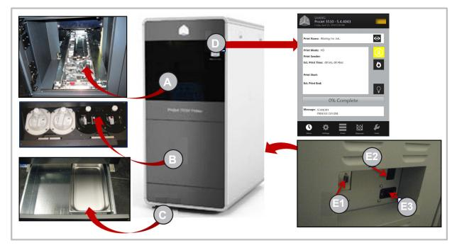
The three dimensional solid parts built by the printer consist of two materials (support material and part material). The support material is a wax based material providing adhesion to build platform, as well as, providing material used to produce supports required to build the model.
