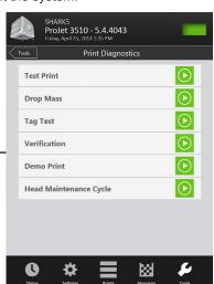
**Printer Diagnostics**: allows you to select the build mode, test a print and perform a demo print.
