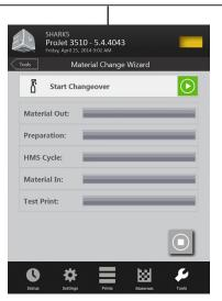
**Material Change Wizard**: if material swap is needed, the change wizard purges the old material out of the printer and performs a test print to ensure the new material is printing.
